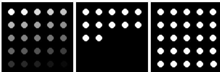
(a) A gradient of grayscales (b) maxValue = 0 and thresh = 127 (c) maxValue = 0 and thresh = 255
